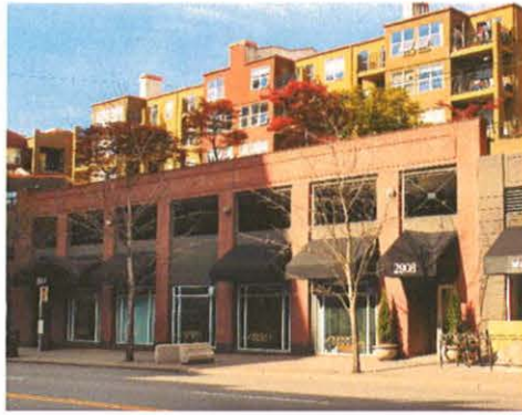
Figure 46. This building uses openings on its second level parking area to resemble windows.
