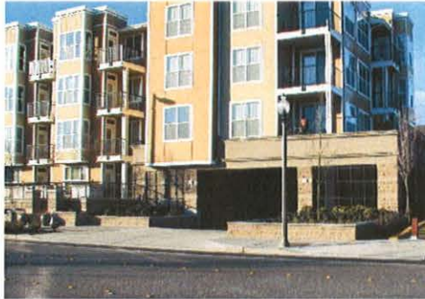
Figure 47. Design parking garages to obscure the view of parked cars. Note the landscaping that separates the garage from pedestrians.
