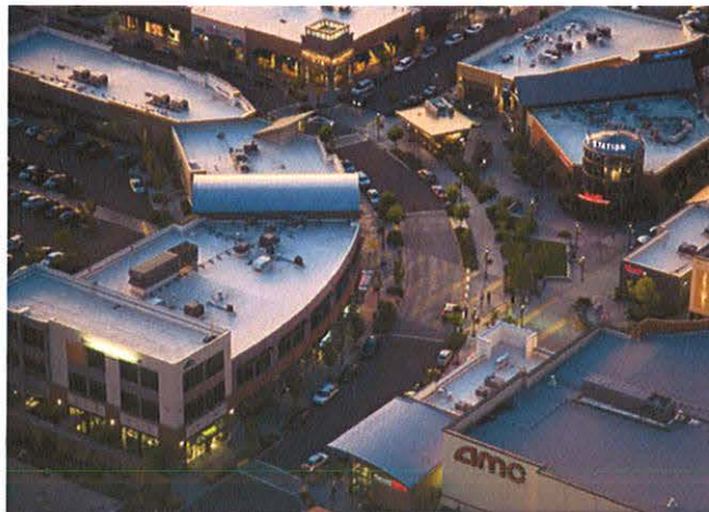
Figure 4. Kent Station internal roadways are one model of internal access roads. Note sidewalks and landscaping.
